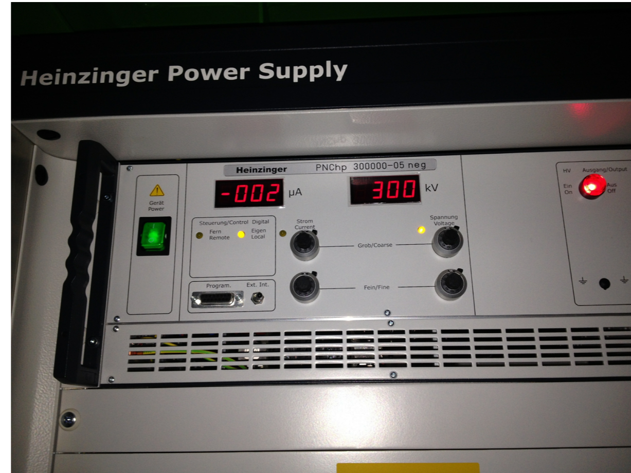
Heinzinger 300 kV Power supply
