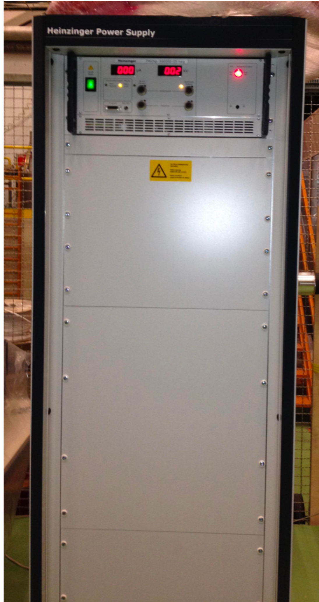
PNChp 300000-05-neg Heinzinger power supply (PSU)
