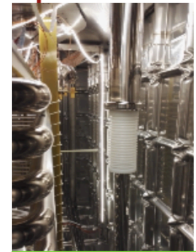
successful test and insertion of 300 kV high voltage feedthrough
