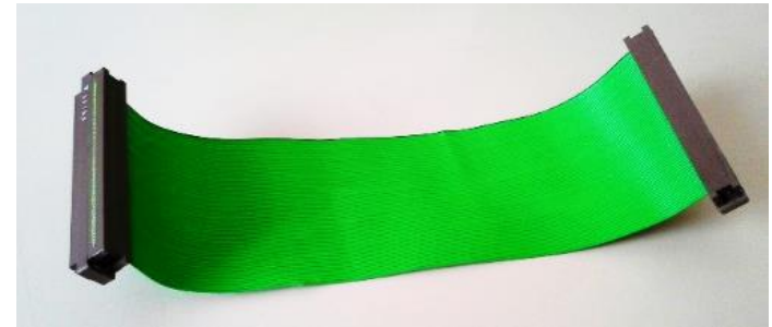
Sample to be tested for continuity in cold and outgassing
