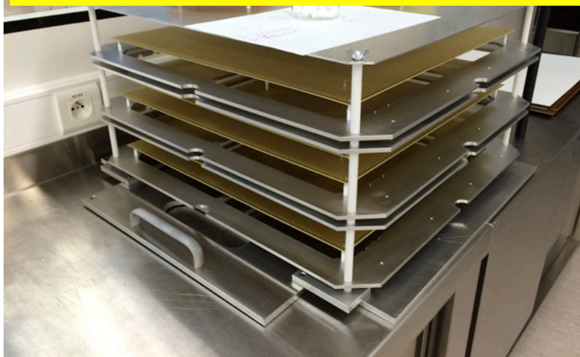
A tower of 6 LEMs can be simultaneously tested in the HP vessel
