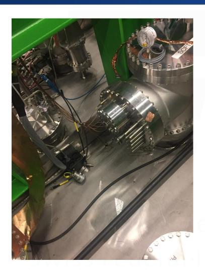
We learnt also more about noise requirement, for example to minimize the noise we had installed copper plates for GND and use some shielded cables to improve the system.
