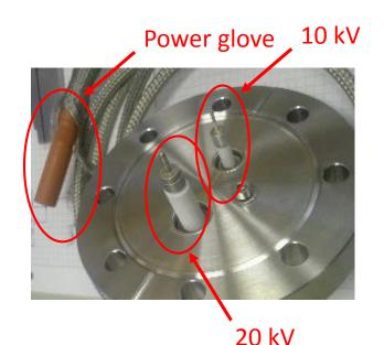
Test flange, with 2 custom made single sided connectors Special silicon cable ("power glove") which evacuates atmosphere around the live pin.
