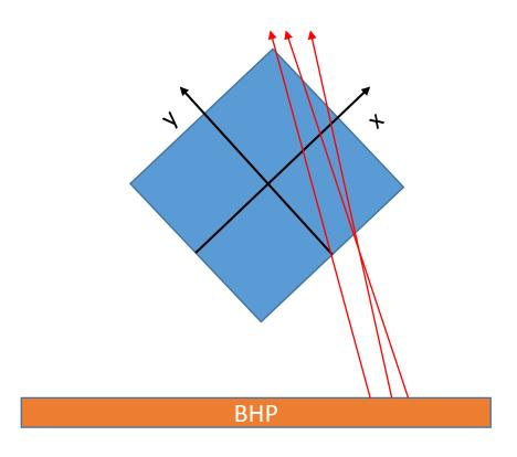
With mean beam position set on the beam right most of the particle trajectories will cross on the positive X side of the CRP
