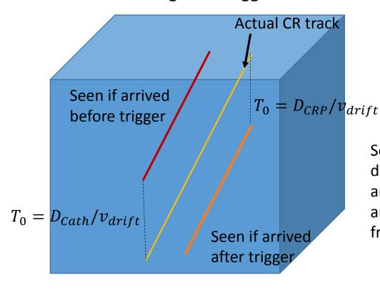
So from endpoints that appear to hang disconnected from either cathode or anode in 3D, we should be able to get  $T_0$  and cross check it against  $T_0$  reconstructed from PMTs
