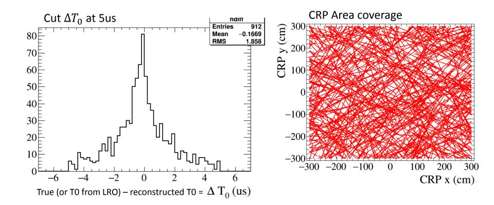
Distribution for 100 simulated CR background events (1s of data taking at 100Hz trig rate) ~900 tracks selected → In principle 9 CR tracks per event for online analyses
