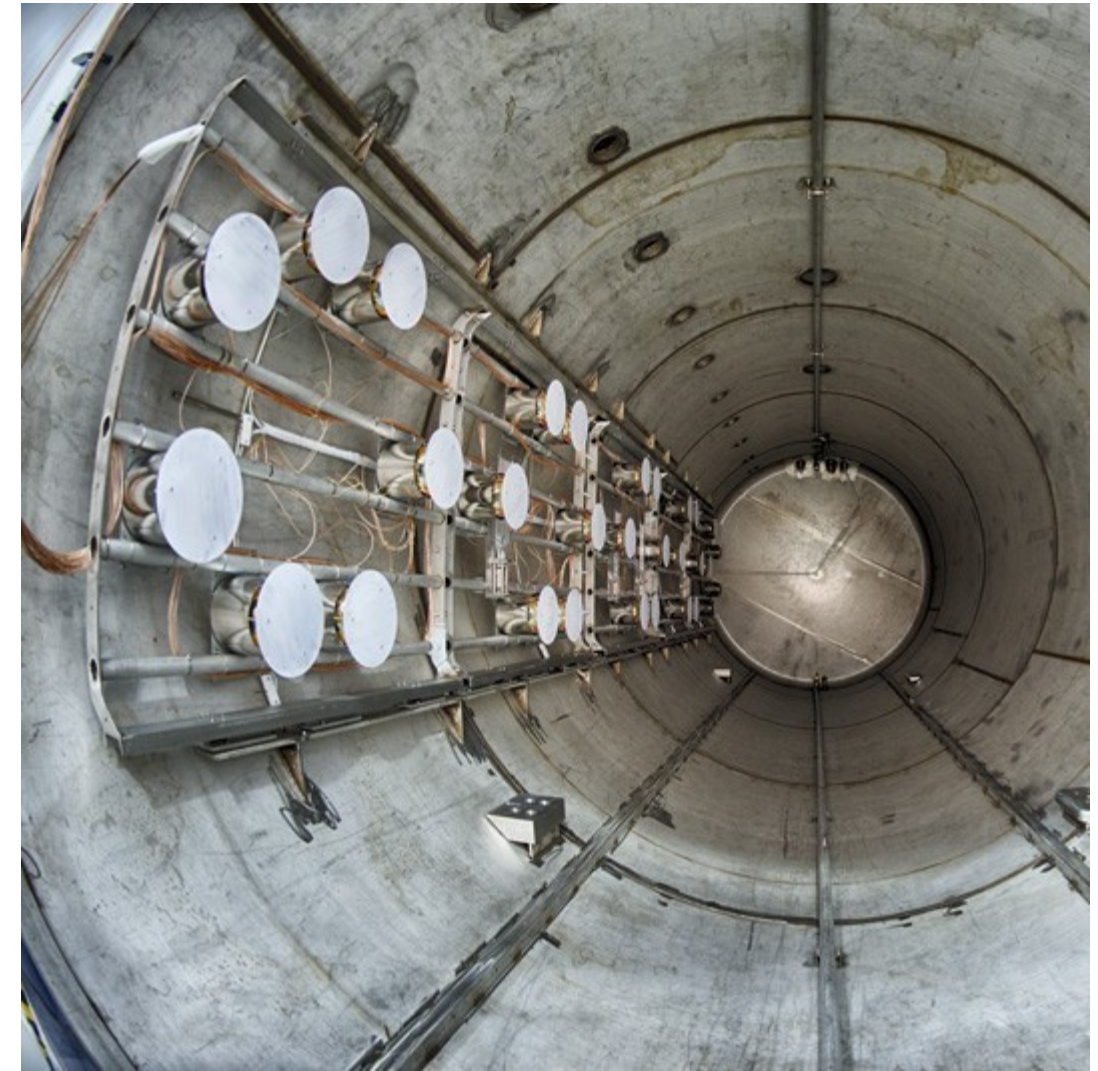
Looking inside cryostat, before TPC inserted
