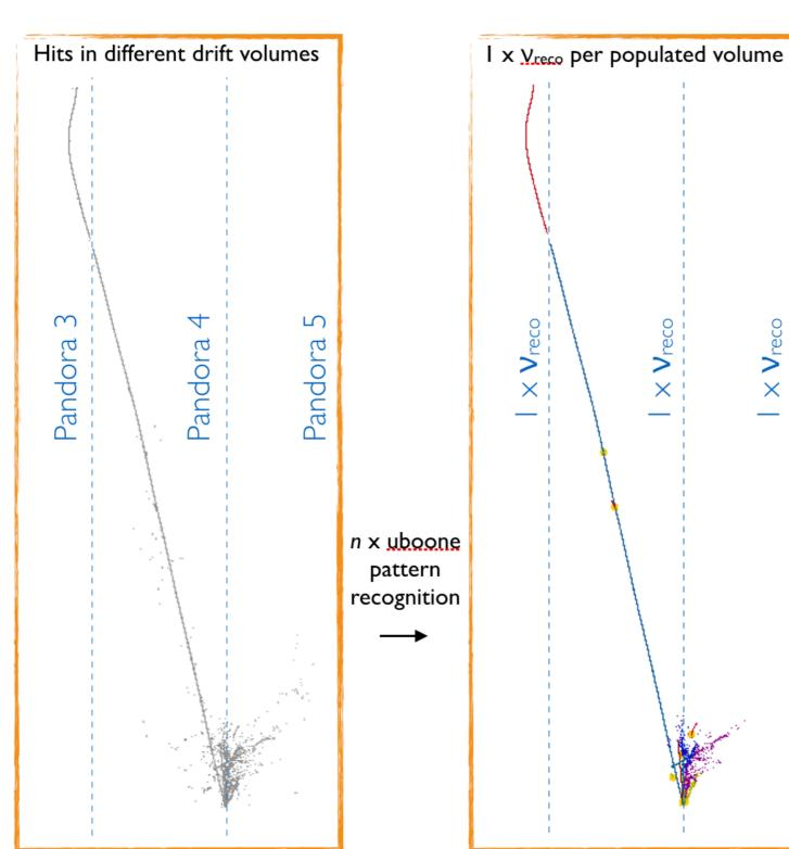
One Pandora per "drift volume": Region with common drift direction, wire pitches and angles.
