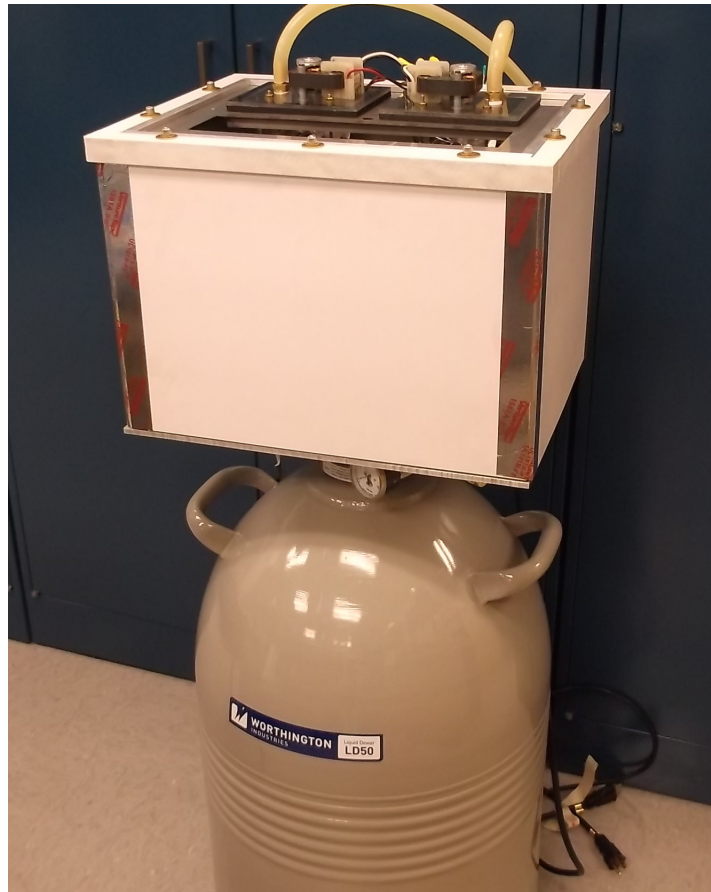
Figure 4: Prototype Cryogenic Testing System (CTS) developed at MSU.
