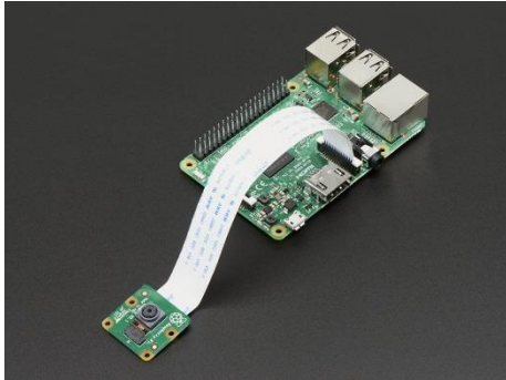
RaspBerry Pi and camera module - 15 pins cable connection
