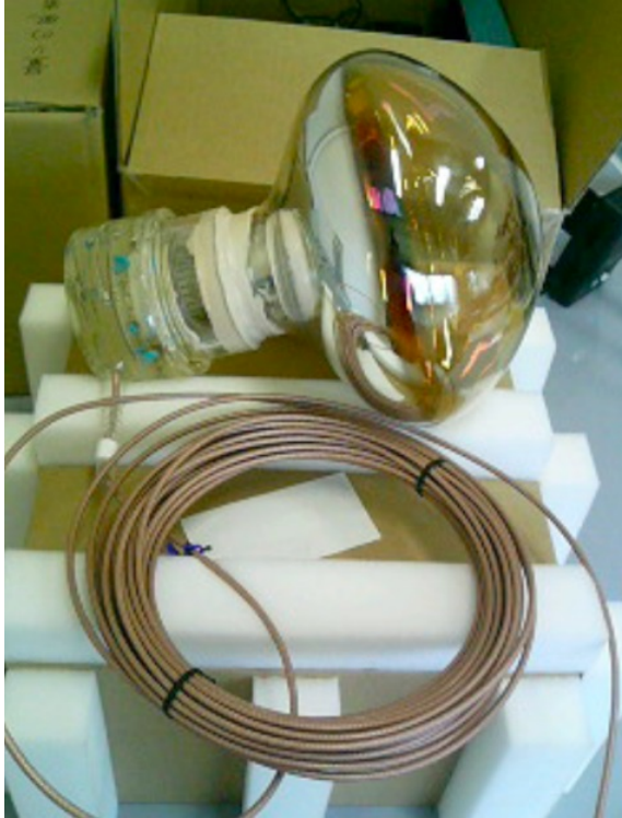
RG-303 attached to a Double-Chooz PMT (external diameter 4.3mm)
