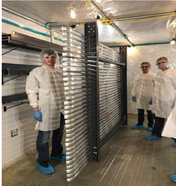
Figure 2: Module-zero completely assembled. The aluminum profiles were precisely aligned at their flat ends during assembly. The alignment of the bent parts in the corner is not representative of the final assembly accuracy since in this pre-production sample the aluminum profiles were not all bent precisely in the same point.
