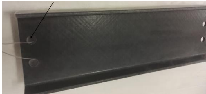
Figure 1: FRP test sample received at CERN for tests at cold and mechanical strength tests
