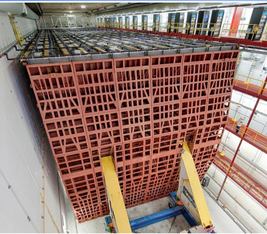
NOvA Far Detector on surface
