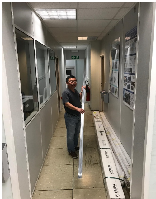
Figure 5 DP FC Field-shaping Profile with a 45 degree bend on one end.
