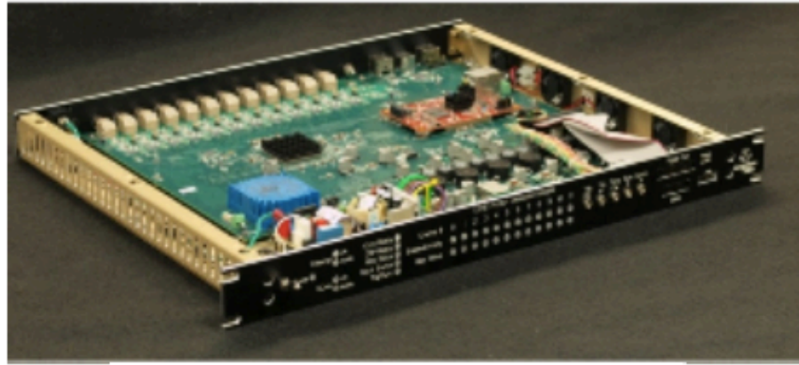
LBNE (DUNE) @ FNAL (35-ton prototype) – Front End Electronics for Photon Detectors Now: 35-ton prototype; Next: CERN TB
