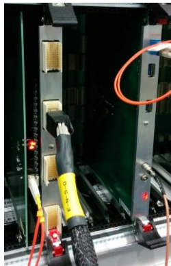
new sPHENIX digitizer prototype
