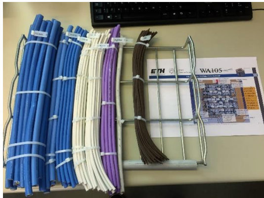
Cable tray 400mm prototyping (without optical fibers).
