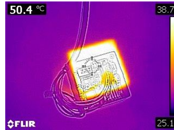
Camera 12V / 0.2A 6W - T° stabilized around 50°C
