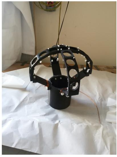
Longer vacuum pumping needed first likely due to plastic outgassing
