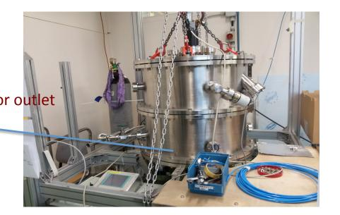
Cristal sensor: measure deposition rate of TPB. Used to checked that all TPB is evaporated
