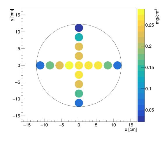
Similar values obtained with Mylar foils (placed in the center of the PMT)
