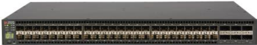
Figure 1: The Brocade ICX 7750-48F features 48 1/10 GbE SFP+ ports and 6 40 GbE QSFP+ ports that can each be split into 4x10 GbE SFP+ ports. The front panel also displays the unit stacking ID.
