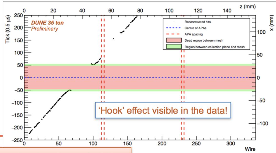
35t APA without the mesh is missing the backwards hits
