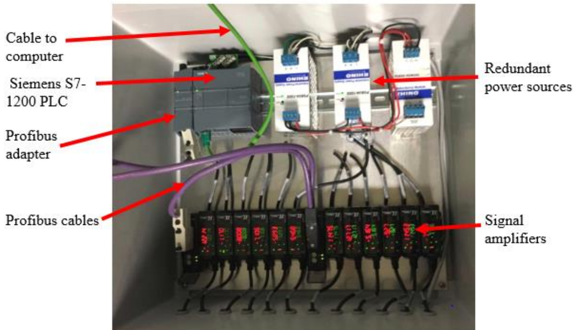
Figure three: Fully assembled equipment housing box
