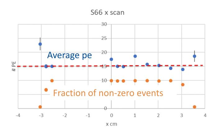
Comment on ave pe: PE itself is not in doubt but to compare to other measurement need to correct SIPM PDE for overvoltage and temperature differences. Studies taken, analysis in progress.
