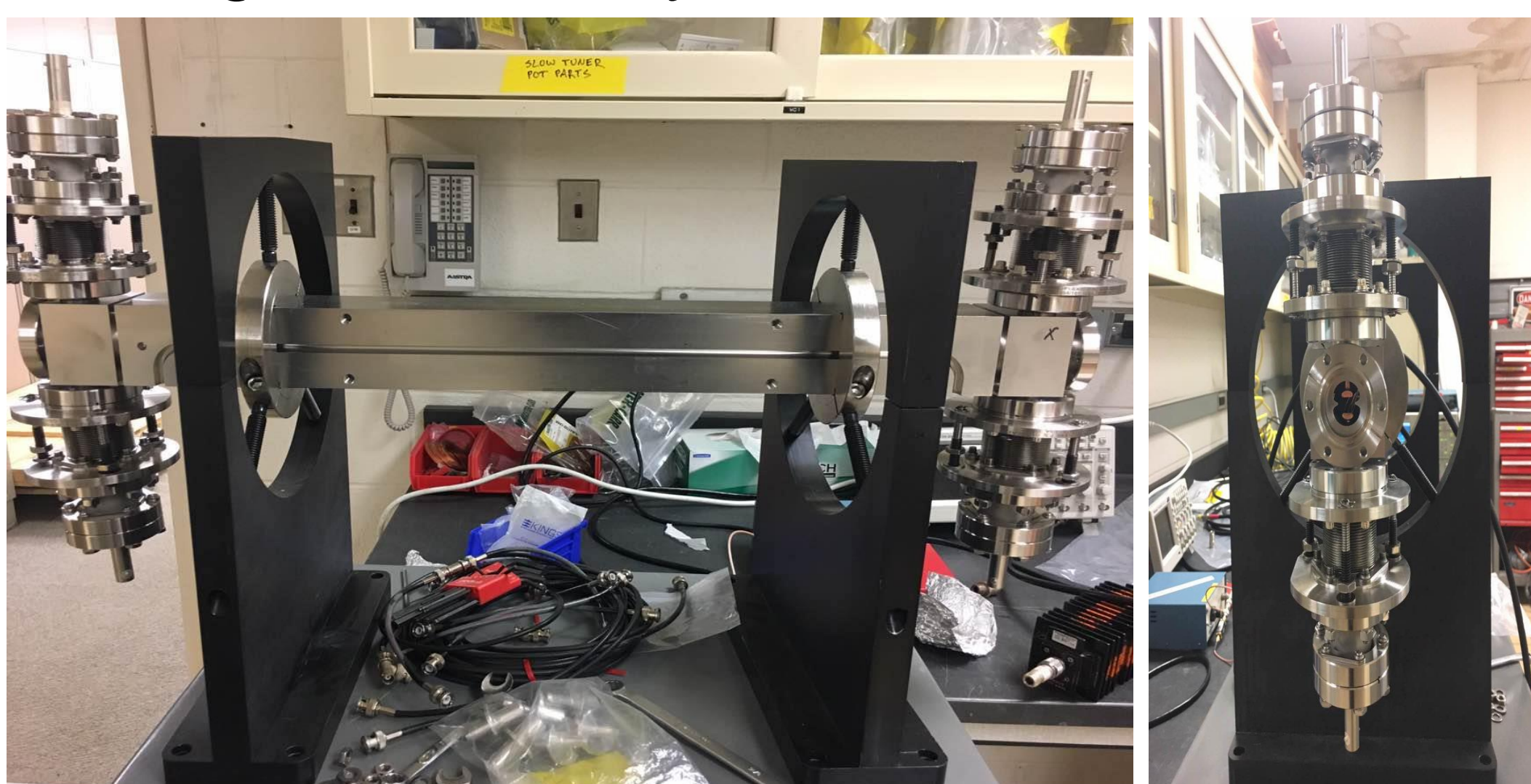
Figure 2: Picture of the transverse stripline kicker at Argonne National Lab, front and side view. (Right) Notice the two copper blades in the middle of the stripline kicker. These are the blades which kicker the beam and will be excited to +/-15 kilovolts in operation with a 22 ns pulse. The blade length is roughly 3/4 meters.
