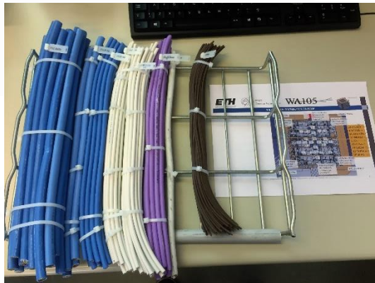
Cable tray 400mm prototyping (without optical fibers).
