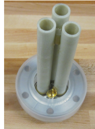
PrM HV/signal feedthrough and brass ground screw
