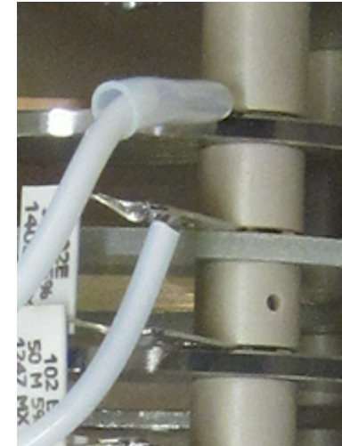
Lugs at anode and anode grid
