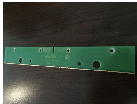
Figure 2.3: top:: illustration of the PCB plates that hold the wires and of the tensioning system on the frame. Bottom: details of the grid HV contact and picture of one PCB wire holder.
