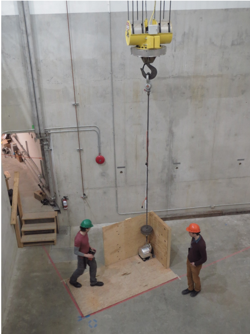
Successful local (pendant controlled) pick-and-place of CERN-ISOLDE-style target vessel onto CERN-ISOLDE-style locating pins using ARIEL Target Hall crane with Target Transfer Tool prototype – 16-March-2018
