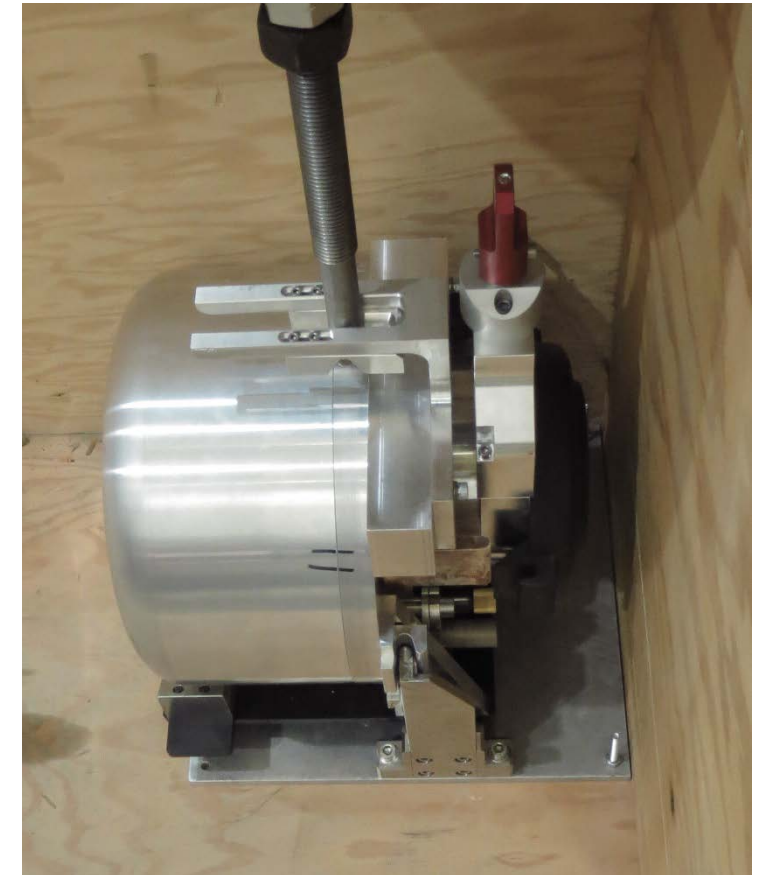
Successful local (pendant controlled) pick-and-place of CERN-ISOLDE-style target vessel onto CERN-ISOLDE-style locating pins using ARIEL Target Hall crane with Target Transfer Tool prototype – 16-March-2018
