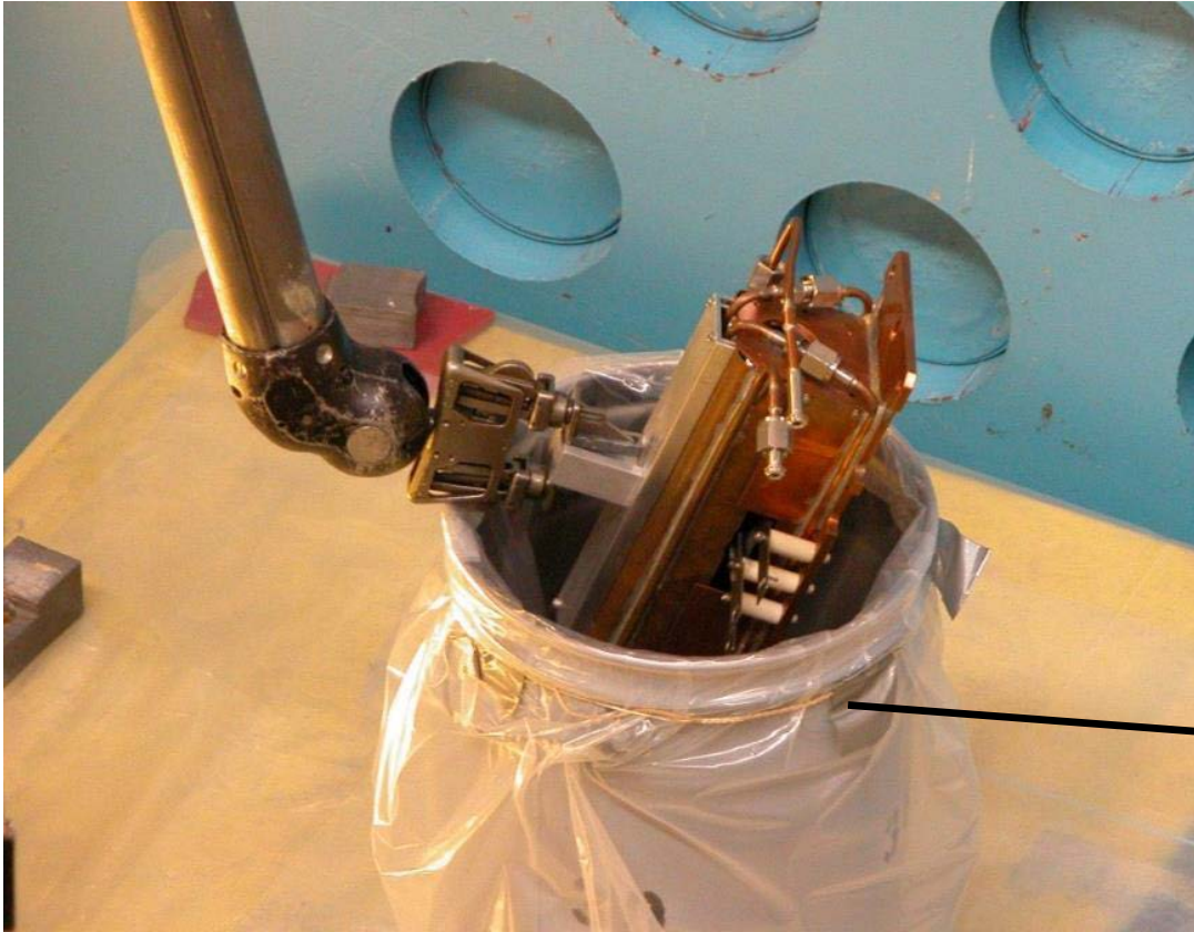
Target loaded into 5-gallon pail in the Hot Cell After decay period , pail is loaded into Nordion F-308 shipping container (manual process!)
