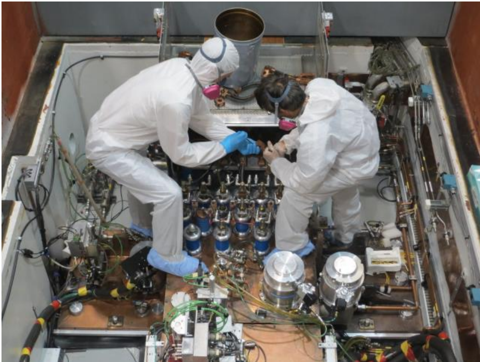
Connecting a Target Module in the pit
