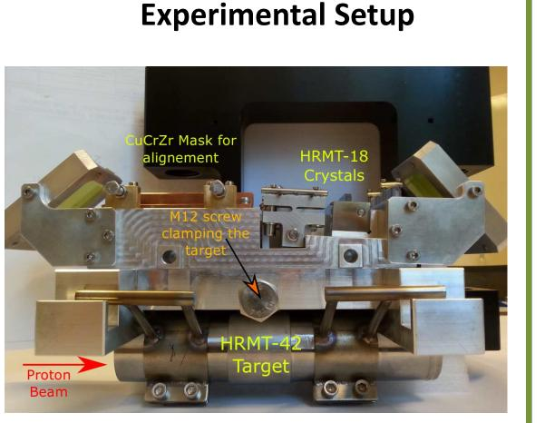
Especially designed robot-friendly clamping system for disassembling the target by just removing one M12 screw
