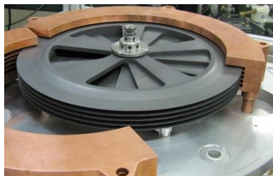
Multi-slice rotating graphite target
