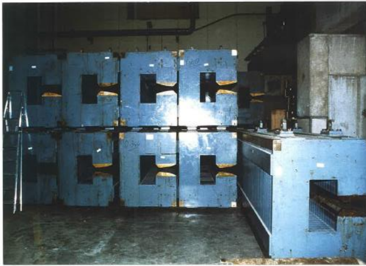
Magnet yokes from the ISR decommissioning
