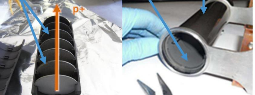
Illustration of an ISOL target SPES Target (INFN Legnaro, Italy) A future target concept that will be used for the 100 MeV PTF would be similar to this one
