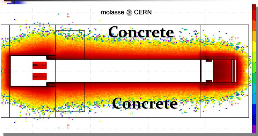
A 6m thickness concrete wall surrounding all the layout limits the production of radionucleides in the molasse. Especially, the production of  $^{22}$  Na and tritium could represent a negative impact by contaminating the ground water.
