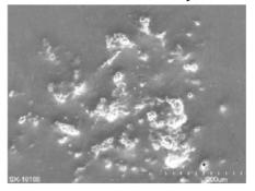
Cavitation damage in wall of Hg target container after 100 pulses of 19 J/cc proton beam (WNR facility at LANL)
