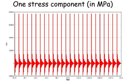
Such results can be used to estimate the fatigue life of the horn
