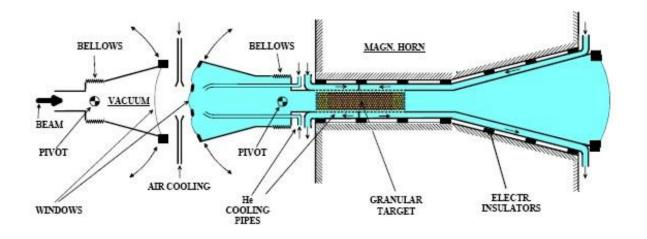
Concept of target integration inside a magnetic horn
