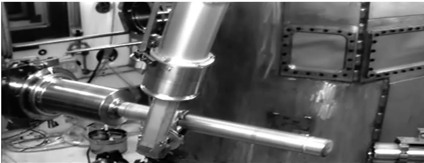
Inspection of the PBW with the flying lead camera
