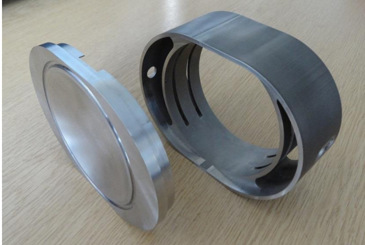
Test piece to develop machining and EB Welding processes
