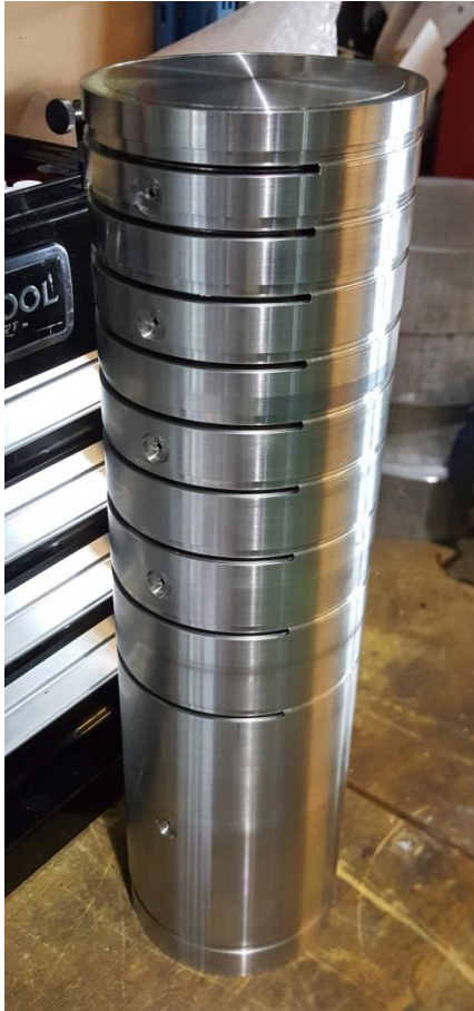
Stack then machined to finished dimensions
