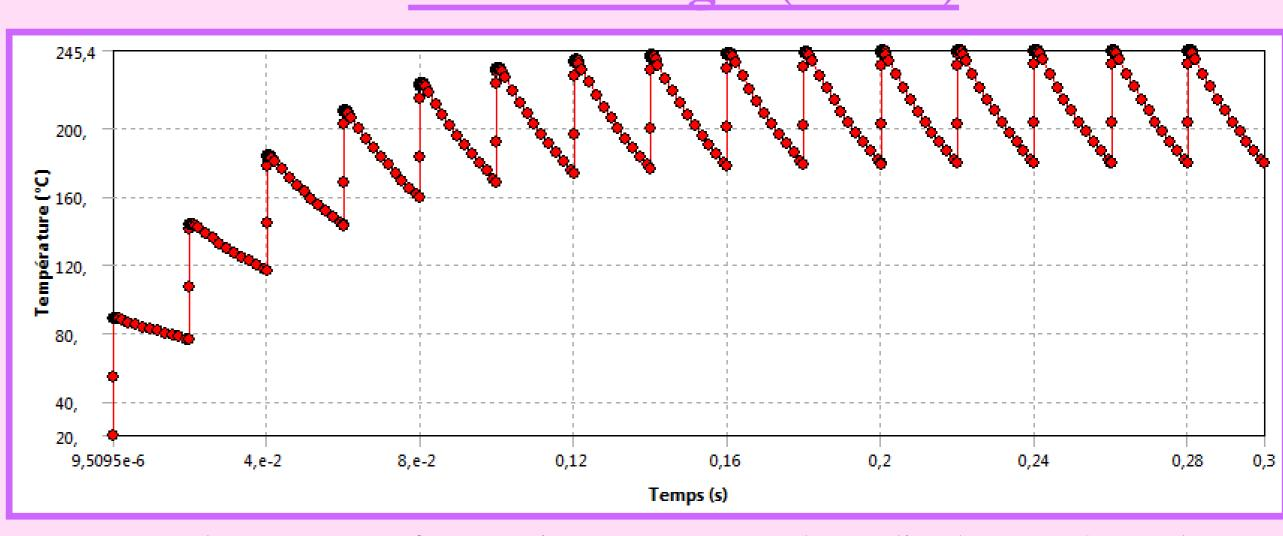
Exemple temperature for a portion target (we see the cooling between 2 rounds)
