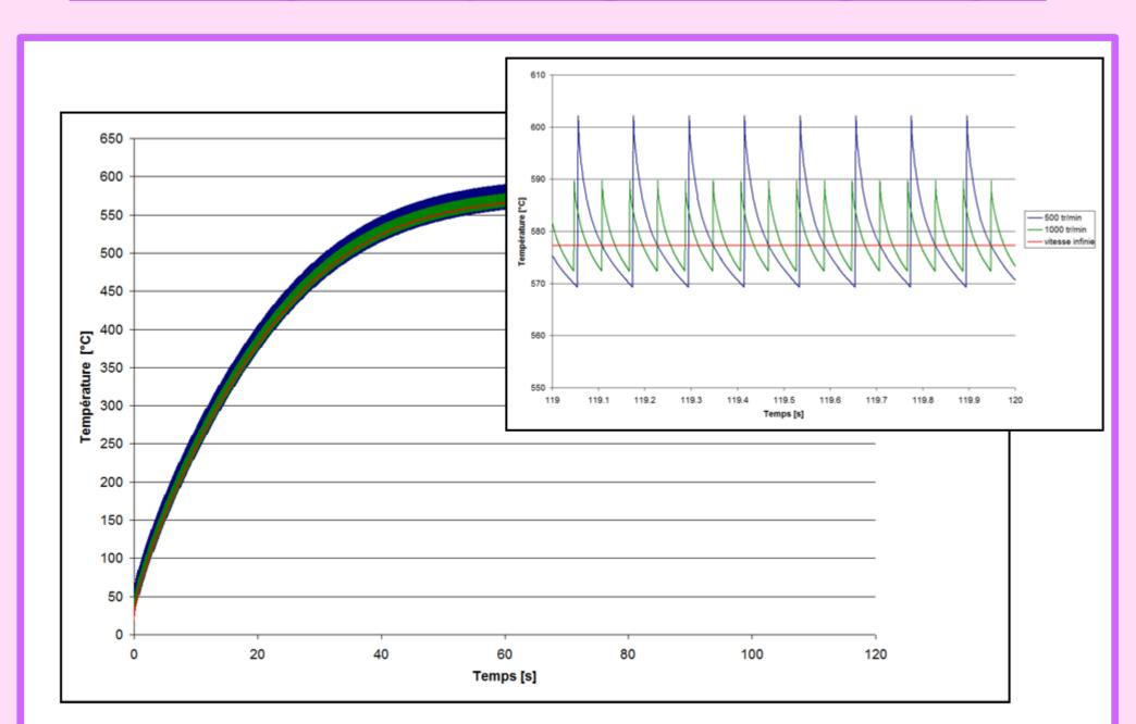
Exemple: temperature depending on the rotational speed for a full target
