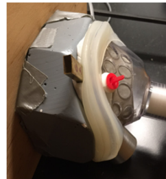
Fig. 2: Picture of leak tube 6A in place between the mask and the mold.
