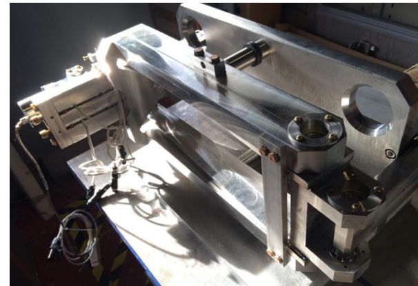
Prototype 650 MHz tuner during bench testing.
