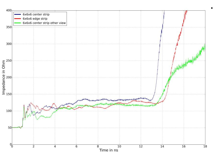
Contacts from connector to strips have slightly different lengths → slightly different durations for signals to traverse entire copper track
