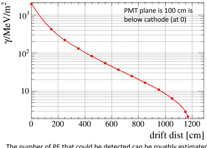
The number of PE that could be detected can be roughly estimated as  $N_{pe} \approx N_d \times 0.0314 \times 0.5 \times 0.2 \times N_{\gamma} = N_d \times 3N_{\gamma}/1000$   $M_{QE}$  Photons / m2 Number of detectors per WLS (1/2 of photons
