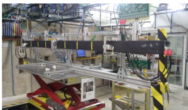
Figure 15: Photo of T-1043 setup showing CRV dicounters mounted on the moveable table.
