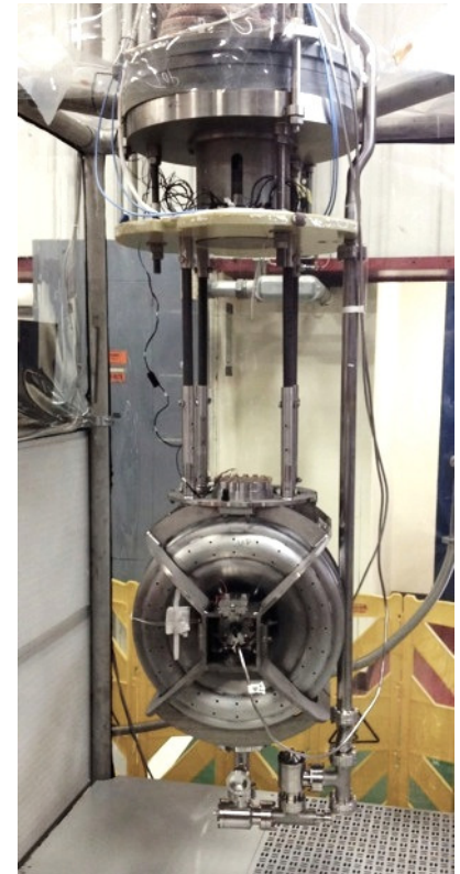
SSR1 cavity – VTS test
