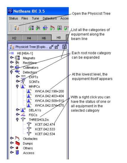
Beam status and settings, equipment status, basic counters, histograms of beam profiles...
