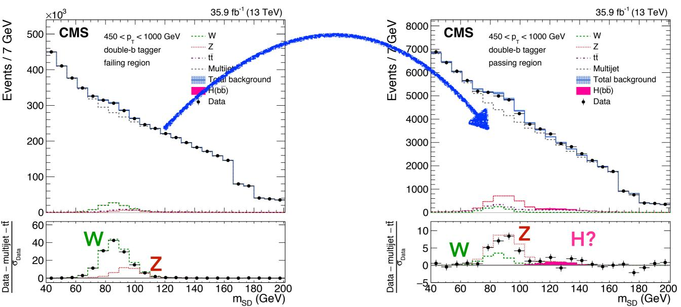
Background prediction in HIG-17-010 proceeds by using taking the m<sub>SD</sub> shape for the QCD prediction from the anti-double-b tagged region modulated by a smooth transfer factor 3
