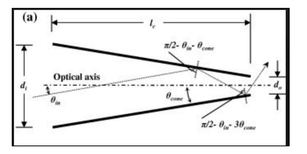
Winston cones are reflective surfaces used to concentrate light from a large area onto a smaller photo-sensitive area.
