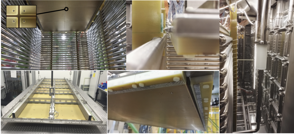
Figure 7: Some details of the TPC. Top-left picture from the drift cage interior looking up to the CRP LEM plane. Top-middle: the top of the drift cage with the CRP and first field shaping ring. Bottom: the CRP during detector assembly top and bottom view. The high voltage feedthrough connected to the cathode inside the cryostat is shown in the right picture.
