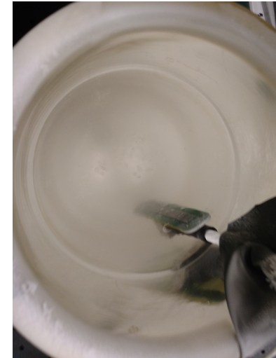
SiPM hoverboard in LN2 for testing SSP noise in cold
