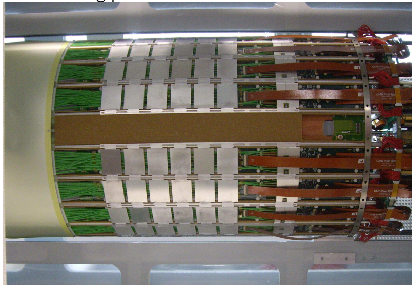
AOH cooling plates
