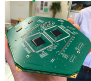
Full module with double-layer PCB readout
